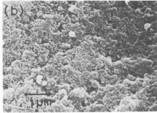
Figure 8 SEM photographs of the fractured surface of shock-compacted bodies which are impacted at a velocity of 2.5 \text{ km sec}^{-1} . (a), (b), and (c) are for initial densities of 30, 50, and 70%, respectively.
